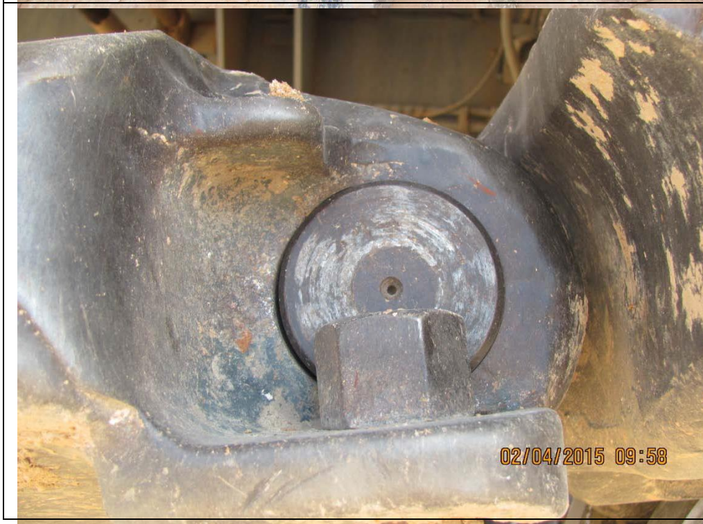
Minimal pin wear on the LH tracks.
