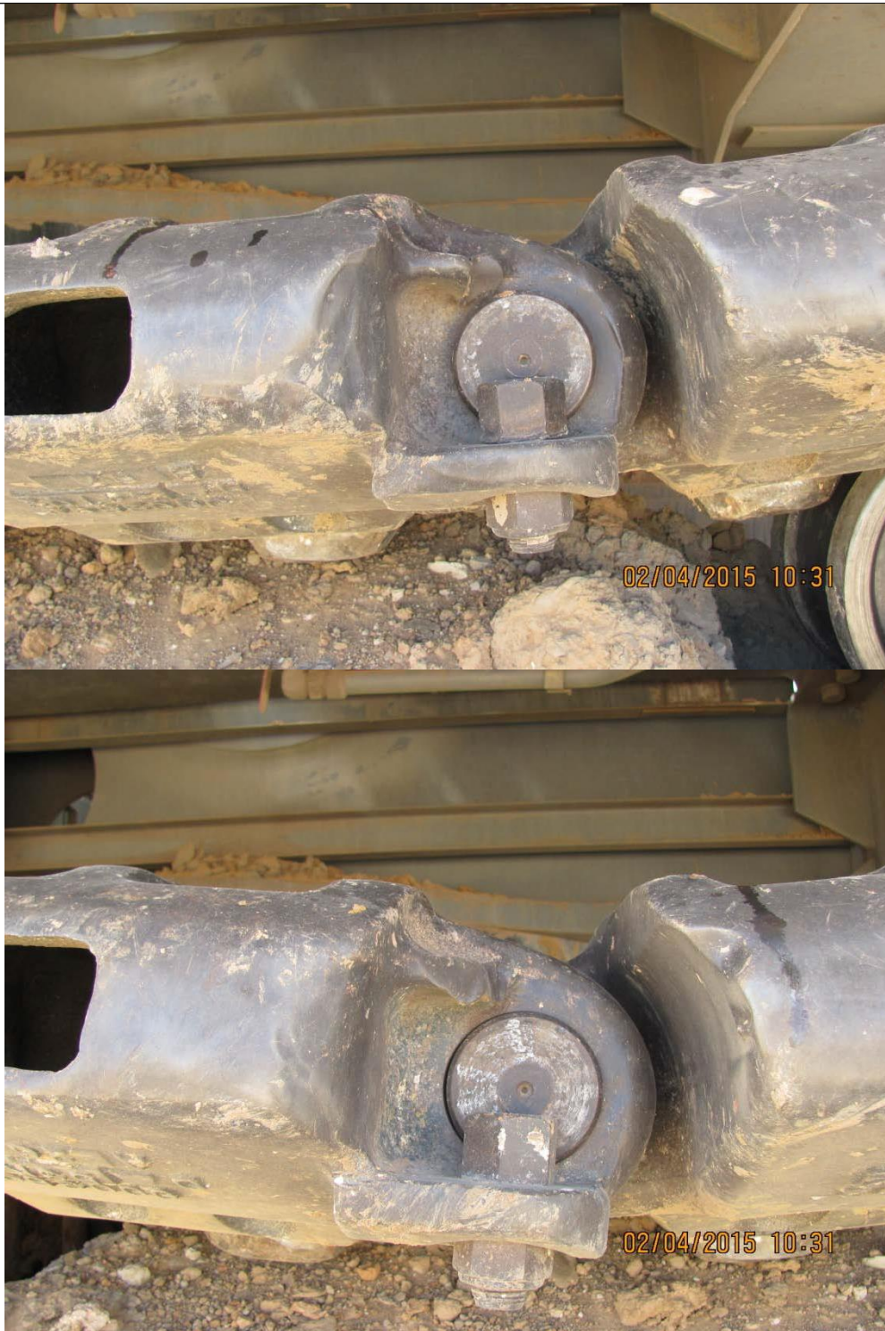
Minimal Pin Wear on the RH tracks
