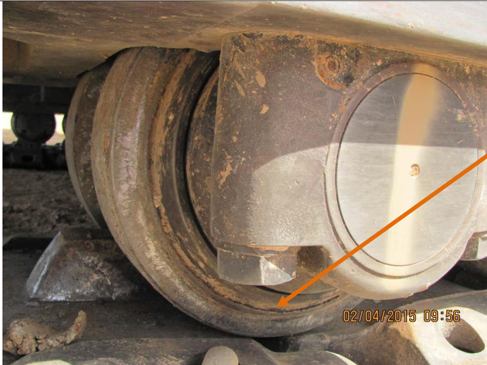
LH Lower Roller 1- outer surface has rolled edges
