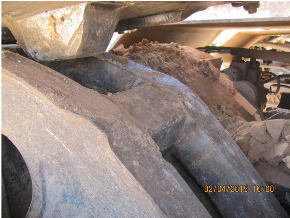
RH Aftermarket Drive Tumbler Profile- Worn outer surface.
