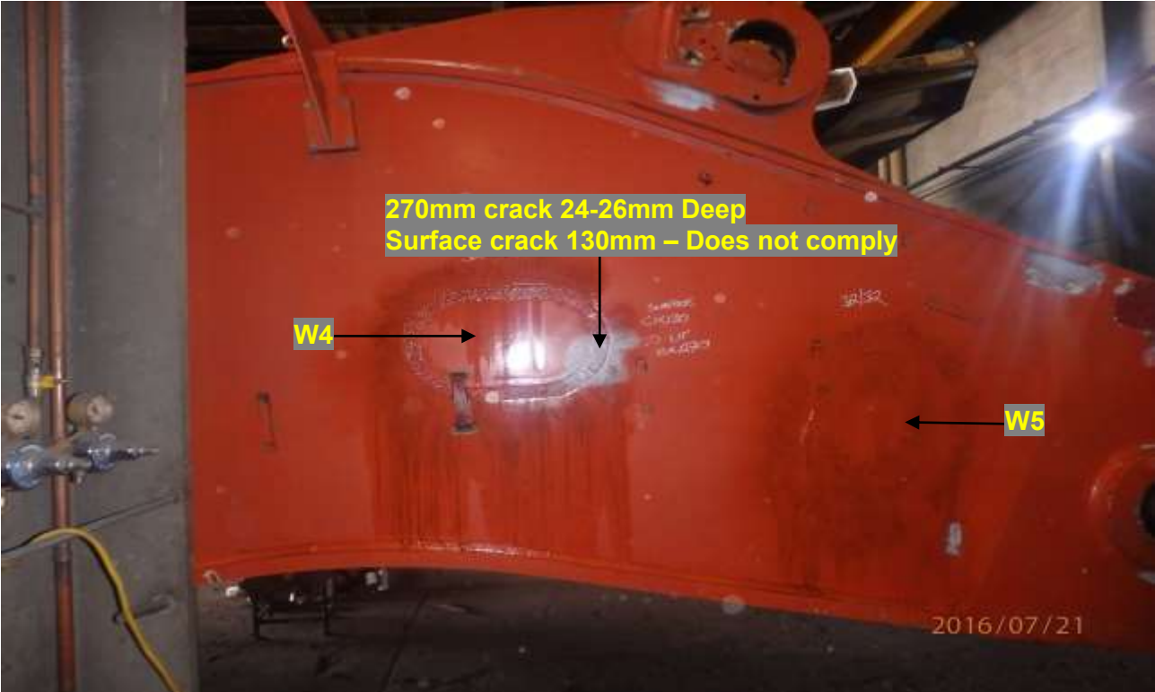
Photograph 1.2. General view of areas examined and discontinuities detected about EX5500 Boom.
