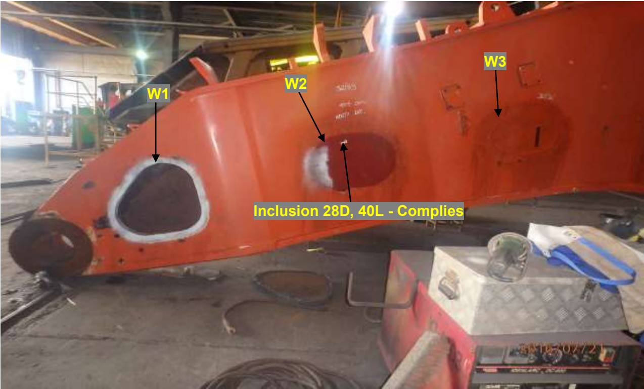
Photograph 1.1. General view of areas examined and inclusions detected about EX5500 Boom.
