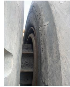
POS 6 SIDEWALL DAMAGE
