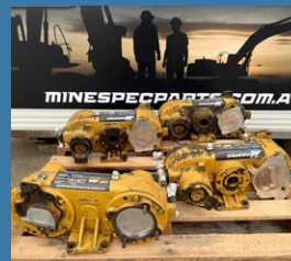
789B PUMP DRIVES
