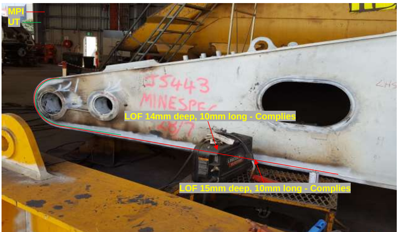
Photograph 1.2. General view of areas examined about Stick, LHS External New Welds JNJ5443
