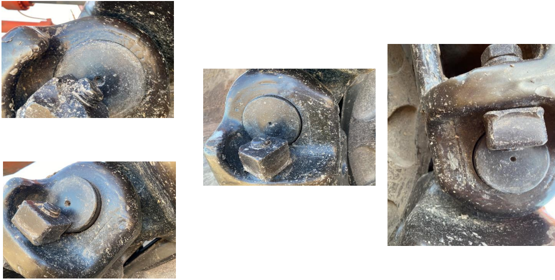
Figure 1 - Typical pin, bore, and retaining hardware condition
