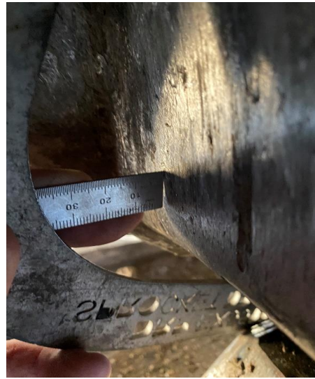
Figure 4 - Sprocket drive lug condition
