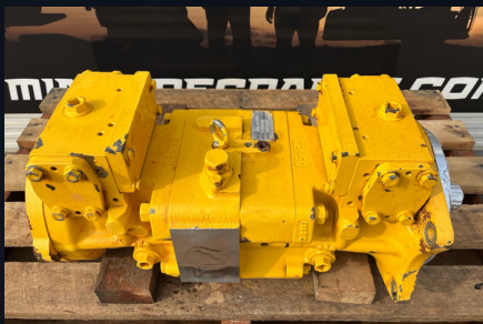
KOMATSU WA900-3EO, SN:60185 PN:708-4L-00931 Pump AS-Steer
