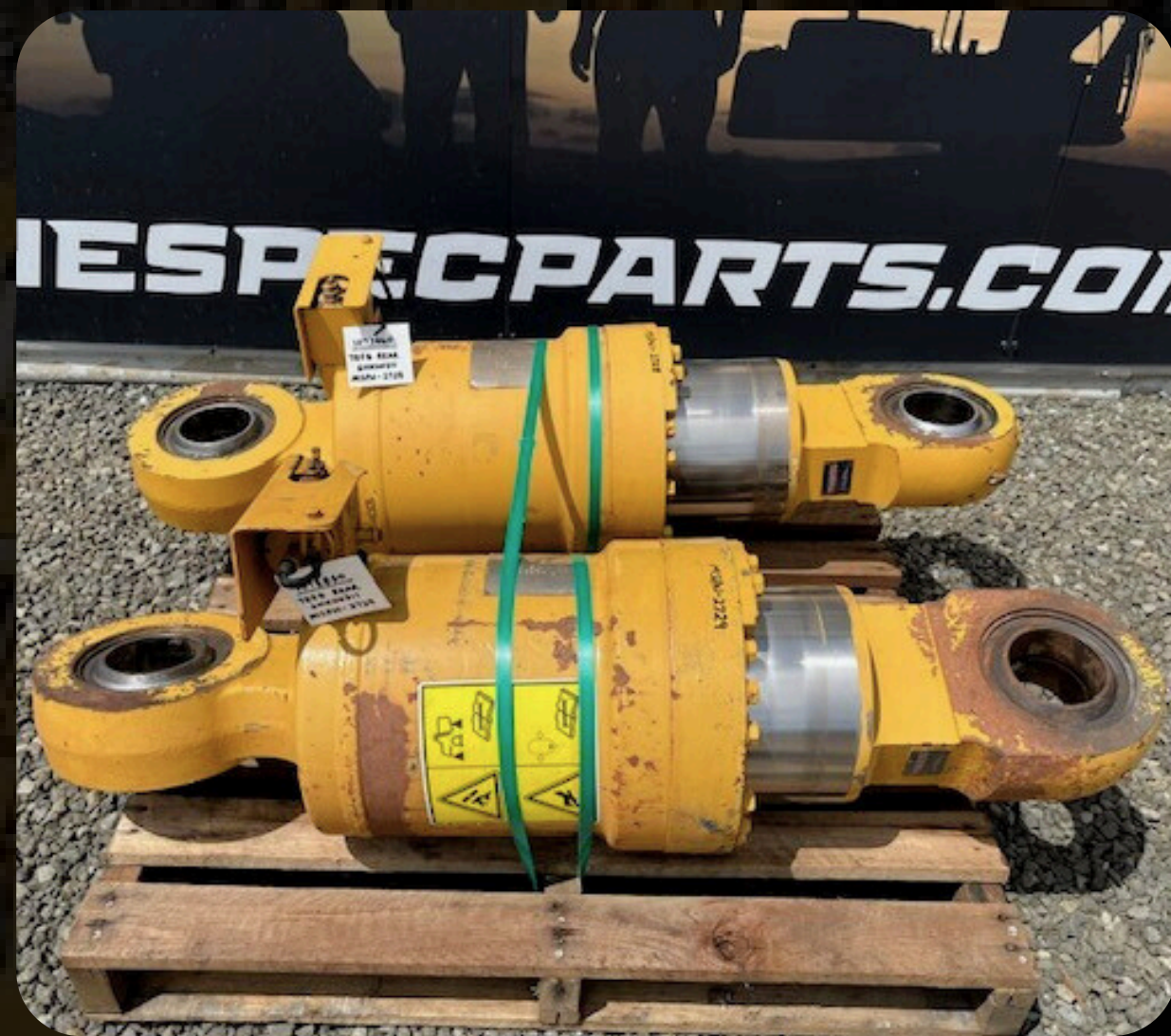
CAT 785C REAR SUSPENSION CYLINDERS PN 1072860
